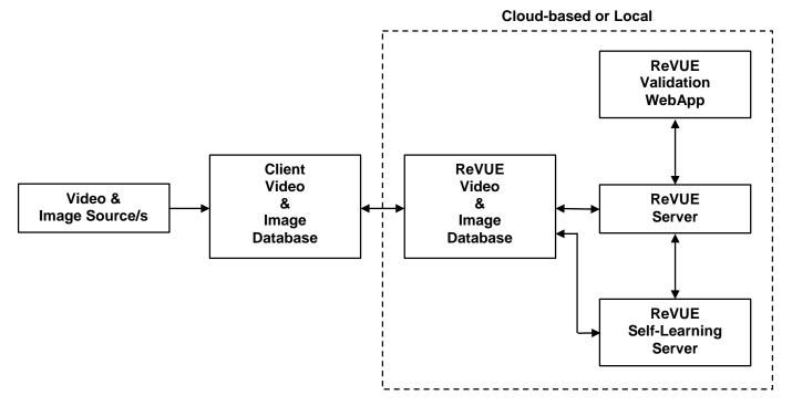
For ReVUE™ implementation, the **Client Video & Image Database** is streamed into the **ReVUE™ Video & Image Database**. The ReVUE™ servers, database and hardware may be hosted in the cloud or locally.
